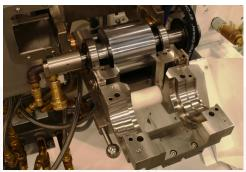
Feed roll bearings feature special seals to minimize silicone contamination and are easily accessed for thorough cleaning. Spare feed rolls and bearings can be provided for quick rotation during material/color changes. This, in turn, enables unprecedented fast change-overs between runs. The extra wide feed opening enhances flexibility for processing.
