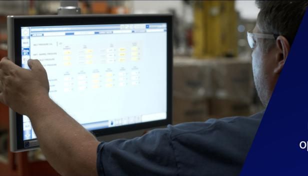
Graham Engineering's exclusive PC-based control system is designed specifically for extrusion and extrusion blow molding machinery. Developed in 2001 as a replacement for traditional PLC-based systems, it provides more flexibility, a higher performance, with a lower cost. The Navigator control system comes in various versions to fit your needs. XC100, XC200, XC300, XBM, and XLS provide varying integration, optimization, and customization levels to your Graham Engineering extruder.
