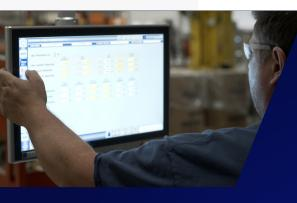
Graham Engineering's exclusive PC-based control system is designed specifically for extrusion and extrusion blow molding machinery. Developed in 2001 as a replacement for traditional PLC-based systems, it provides more flexibility, a higher performance, with a lower cost. The Navigator control system comes in various versions to fit your needs. XC100, XC200, XC300, XBM, and XLS provide varying integration, optimization, and customization levels to your Graham Engineering extruder.
