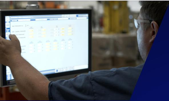
Graham Engineering's exclusive PC-based control system is designed specifically for extrusion and extrusion blow molding machinery. Developed in 2001 as a replacement for traditional PLC-based systems, it provides more flexibility, a higher performance, with a lower cost. The Navigator control system comes in various versions to fit your needs. XC100, XC200, XC300, XBM, and XLS provide varying integration, optimization, and customization levels to your Graham Engineering extruder.
