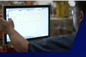
Graham Engineering's exclusive PC-based control system is designed specifically for extrusion and extrusion blow molding machinery.
