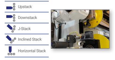
Highly efficient & maintenance-friendly heat/cool systems control the temperature of the chrome rolls with nips that are controlled hydraulically, pneumatically, or by boosted pneumatic. Key features of the take-off include automatic functions for critical product quality attributes such as roll skewing, crowning & electronically-controlled gap adjustment.
