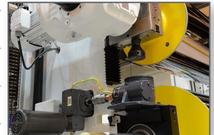
Highly efficient & maintenance-friendly heat/cool systems control the temperature of the chrome rolls with nips that are controlled hydraulically, pneumatically, or by boosted pneumatic. Key features of the take-off include automatic functions for critical product quality attributes such as roll skewing, crowning & electronically-controlled gap adjustment.
