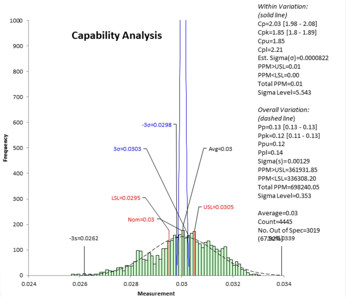
This process is out of control and would require a tolerance a decade higher than the  $\pm 0.0005$ " (and still would not pass validation efforts). Data within each subgroup of 5 readings (short term, 2.5s or 1.6 ft of tubing) was certainly not horrible, but the overall long-term performance of the process was. Note the Xbar/R charts on the next page.
