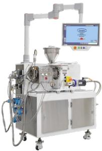
Extruder - Graham Engineering modular extruder with Navigator X200 controls,  $\frac{3}{4}$ " barrel module, single flighted 17-4 screw with 40-60-80-200-40 screens and a Beckhoff 8.2Nm servo.
