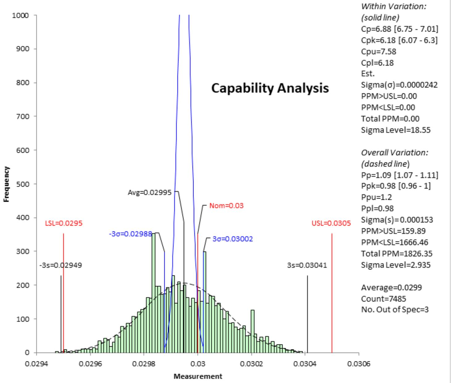
With the pressure control enabled, the variation with subgroups tightened considerably. Long term Pp and PpK also increased substantially. The only drawback to this feed throat design is that the process solids conveyance failed completely 2 times before data could be collected continuously for an hour and failed a 3rd time not long after the experiment was completed.
