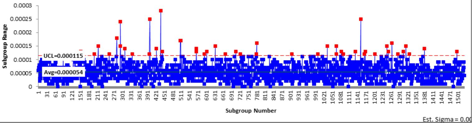
The UCL and average for the R chart is reduced significantly from the standard 2 grooved feed insert. Some outliers noted due to water on the tubing found in the collection tray (not removed from the calculations).
