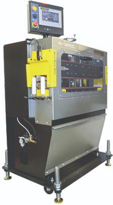
Puller/Cutter - Novatec Servo Controlled puller/cutter set to 95 FPM
