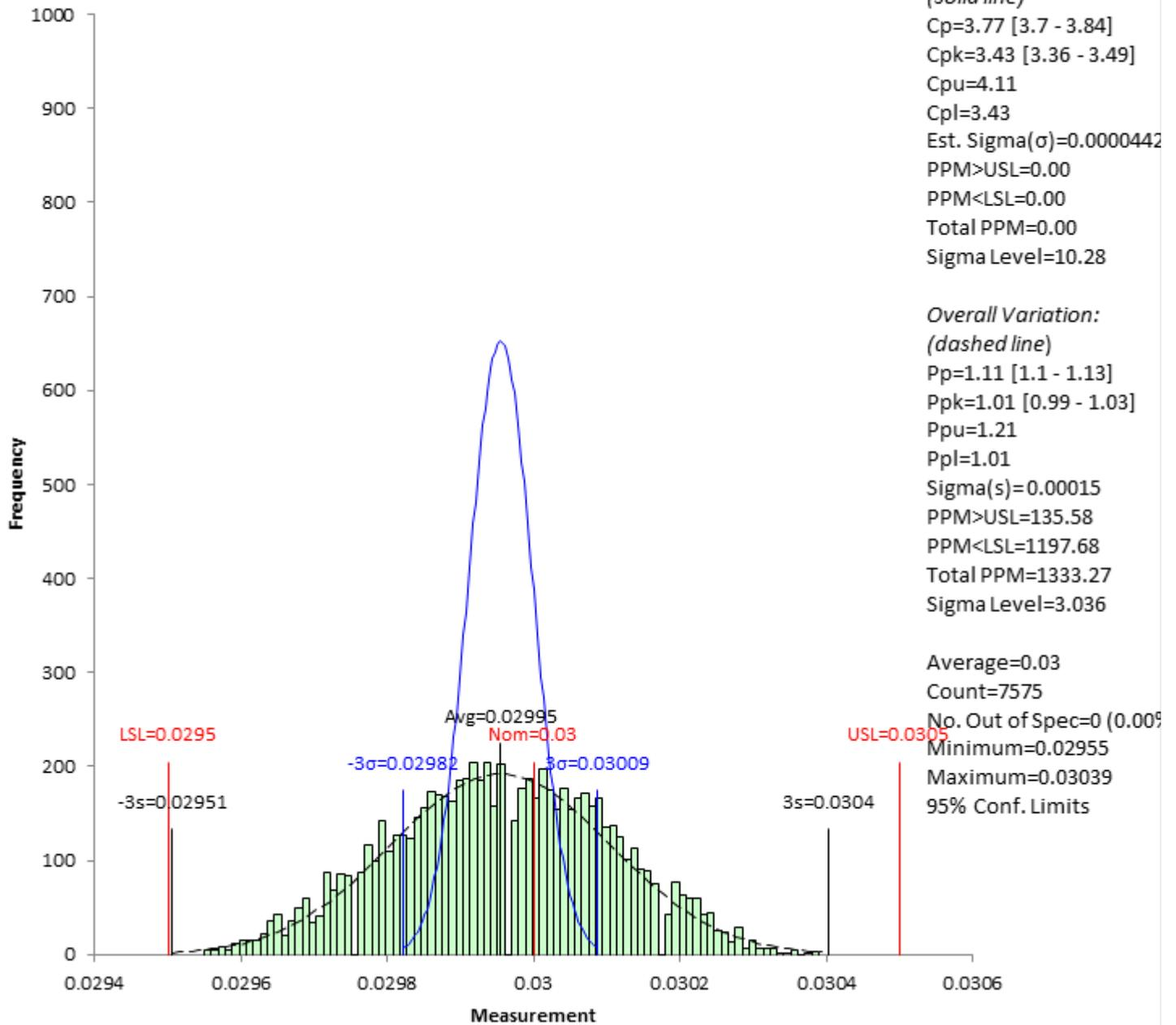
For this experiment, the variation within the subgroups increased over the smooth bore design, though the Pp and PpK are similar to the smooth bore insert (modest gain).
