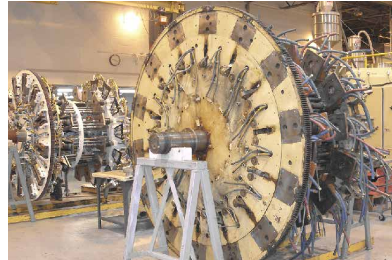
Graham Engineering® rotary wheel spools before (foreground) & after (background) a major rebuild. Minor rebuilds are used to maintain your machine in peak running condition, while major rebuilds are used to obtain “like new” performance.
