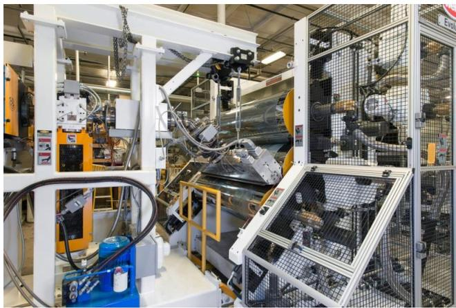
In 2017, Pro Ex partnered with Graham Engineering to specify a Welex Evolution sheet line that would expand its capability and capacity. Commissioned in December 2017, the dual-resin PET/PP line features a 5" (130 mm) extruder with the flexibility to expand to co-extrusion. The J-stack configuration features roll-skewing and electric gap adjustment under full hydraulic load followed by a unique arrangement of auxiliary cooling rolls, each independently driven, heated, and cooled.
