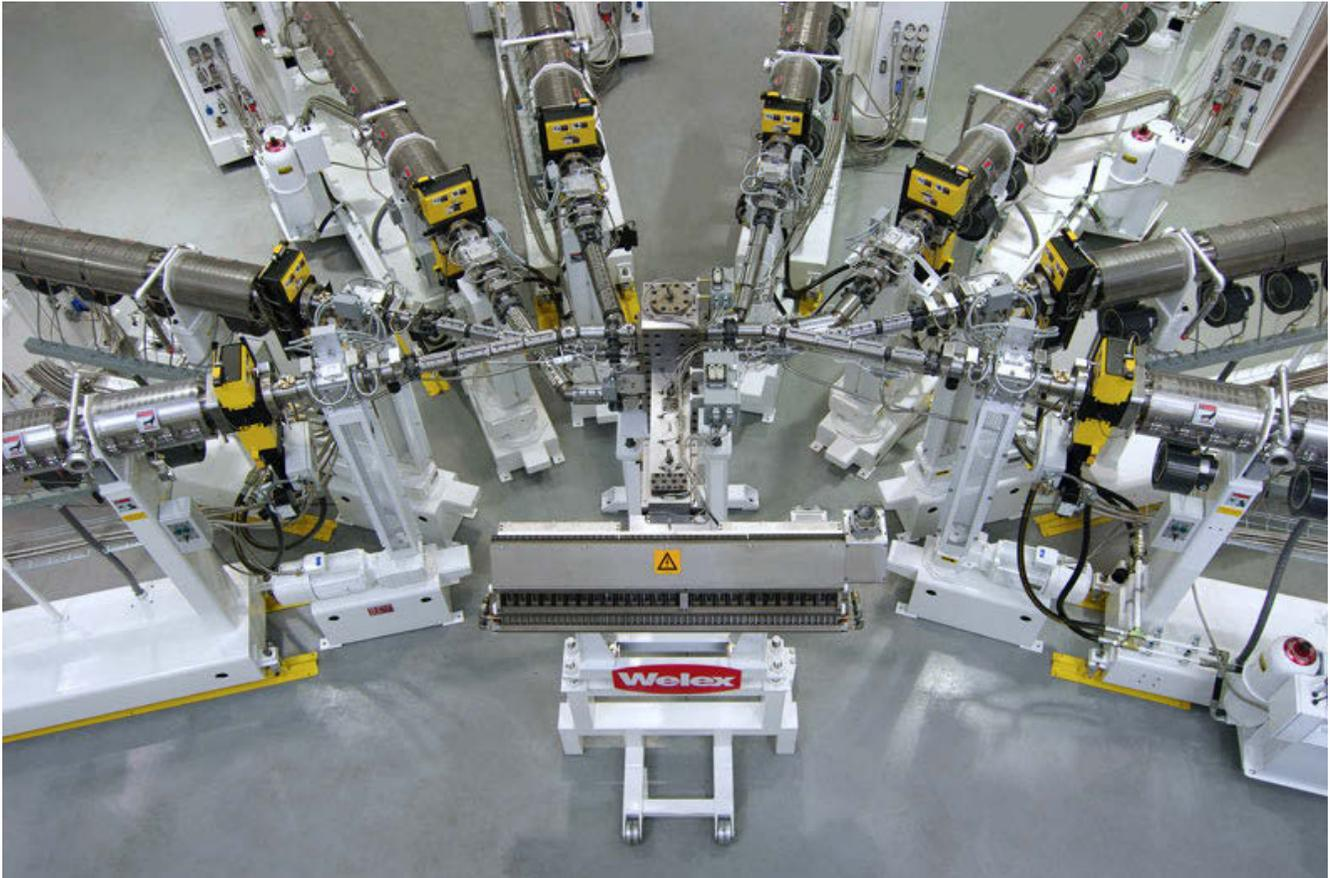
Caption: Welex Inc.'s new custom nine-extruder, five-layer sheet extrusion system is for the production of multi-colored striped sheet for thermoformed yogurt cups. Overhead ninth extruder is omitted from photo.
