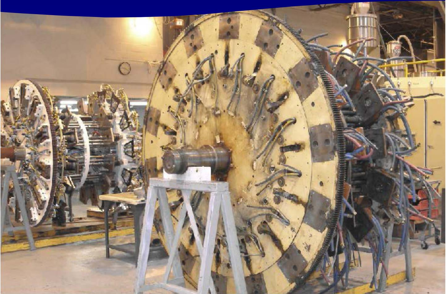
Graham rotary wheel spools before (foreground) and after (background) a major rebuild. Minor rebuilds are used to maintain your machine in peak running condition, while major rebuilds are used to obtain “like new” performance.
