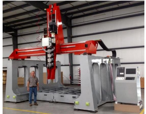
*Thermwood's 3D Additive Manufacturing System initial development machine can make parts up to 10'x10'x5'*
