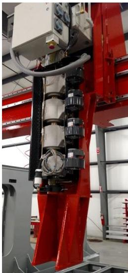
*The system's 1.75" vertical extruder from American Kuhne is fully integrated to provide precise material distribution*
