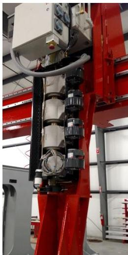
*The system’s 1.75” vertical extruder from American Kuhne is fully integrated to provide precise material distribution*
